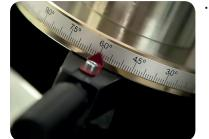
Support pins to fix the angles at 45° and 90°' degrees.
