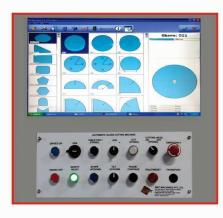
Automatic Cutting pressure adjustment when you choose glass thickness to cut. There is a recipe provided in the software, which chooses right cutting pressure for right thickness of glass automatically.
