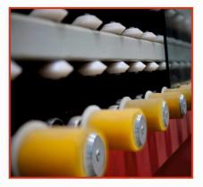
Conveyers have Special Rollers made of Poly Urethene which has long life and very easy to change. Conveyer Speed has a speed controller which is used to increase or decrease the speed.
