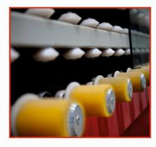
This panel press line is capable to work with warm edge spacer bar technology and aluminum or plastic spacerbar. To apply warm edge spacer tilt table is used and to apply aluminum spacer bar assembly table is used which is shown in the picture on the right side Conveyers have Special Rollers made of Poly Urethene which has long life and very easy to change. Conveyer Speed has a speed controller which is used to increase or decrease the speed.
