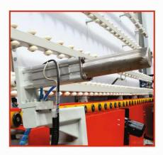
Glass thickness is measured along with spacer bar gap at this point immediately after the unit comes out from the panel press line. The spacer bar thickness gives a signal to the sealing robot how much flow rate of silicon to be kept while sealing. This flow rate comes from the recipe which is stored in the PLC software.
