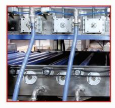
Washing and drying section can move upwards which gives enough space for operator to clean the machine inside.
