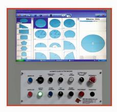
Automatic Cutting pressure adjustment when you choose glass thickness to cut. There is a recipe provided in the software, which chooses right cutting pressure for right thickness of glass automatically.
