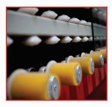
Conveyers have Special Rollers made of Poly Urethene which has long life and very easy to change. Conveyer Speed has a speed controller
