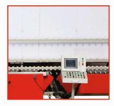
The outlet rack is divided in two parts which enables one piece of glass being sealed while other is waiting on the final outlet rack to be unloaded. This gives a better production capacity. Touch screen on the control panel
