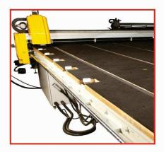
Automatic Glass transfer from Loading Table to Cutting Table and then to Breaker bar table by transport belts.
